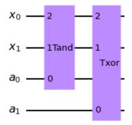
Now, transform the irreversible circuit for the two-bit adder above to a **reversible** circuit C for the two-bit adder. More precisely, the circuit C should act on bits
